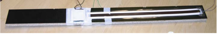
Fig. 2. The CheapStick was built with pressure sensors made from a porous material and a position sensor made by video tape
